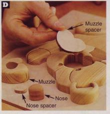
Install the muzzle spacer followed by the muzzle. Then insert the nose spacer and the nose into the muzzle opening.
